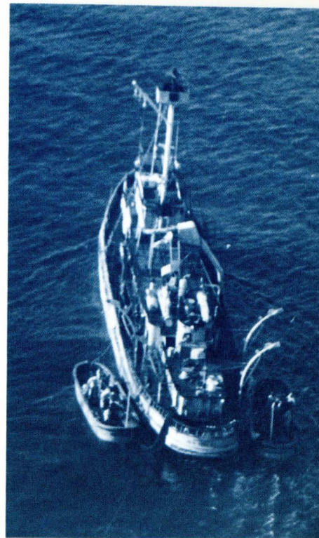
The menhaden trawler lowers her two purse boats and puts aboard the seine between them.
