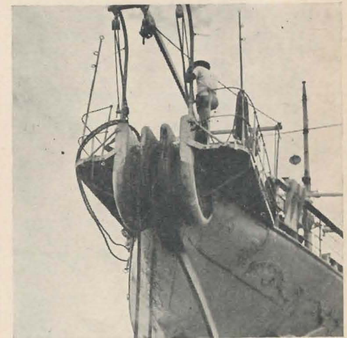
OVER THE BOW —This is the bow of the Restorer with its large cable sheaves, shown as it reels in two separate cables; a rare feat for a vessel used in this type of work. Powerful grappling hooks are strung over these grooved wheels when the ship is dragging the ocean bed in search of the cable.
