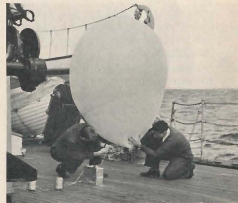
Photo by Commander R. B. Hall U. S. Coast Guard Cutter " Pontchartrain " Attaching radio sound transmitter to balloon. This apparatus transmits signals indicating humidity, temperature and pressure which are intercepted by the weather observer on the ship. An average run of this balloon will reach approximately 22,000 meters.
