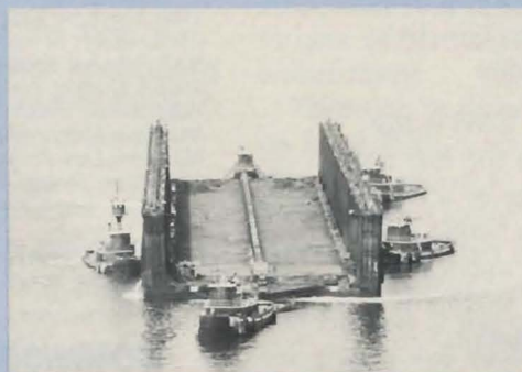
Five tugs were required to move this 700 foot-long floating drydock across New York harbor from a berth in Jersey City, New Jersey to a new location in Brooklyn, New York.
