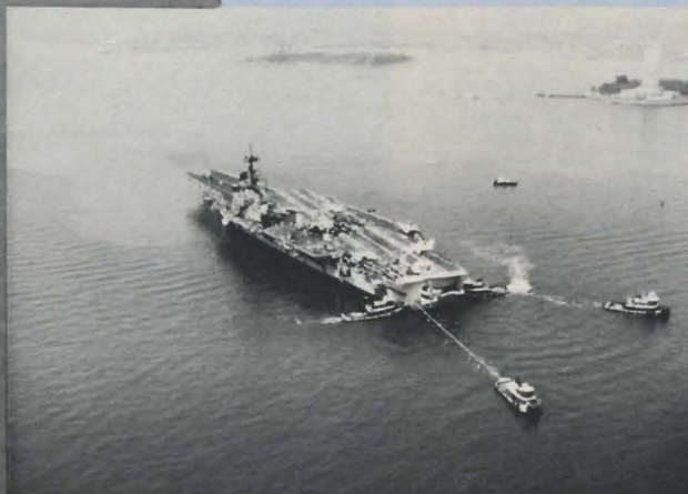
When the USS Independence visited New York harbor last year, four tugs held the aircraft carrier on station at its anchorage near the Statue of Liberty.
