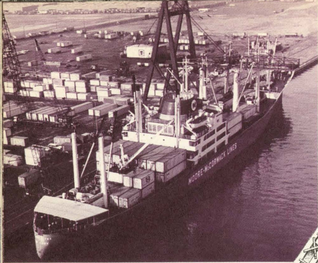
◀ Containers are stowed above decks on some vessels.
