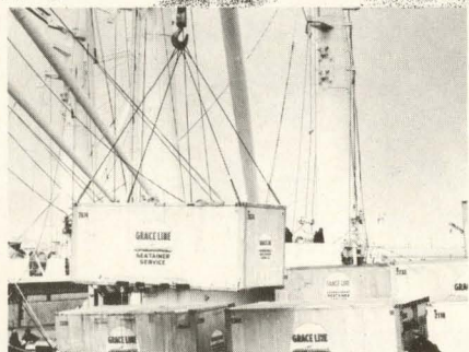
◀ Some of the newest container ships have their own built-in gantry cranes which are adaptable for operation on either the port or starboard sides of the ship.
