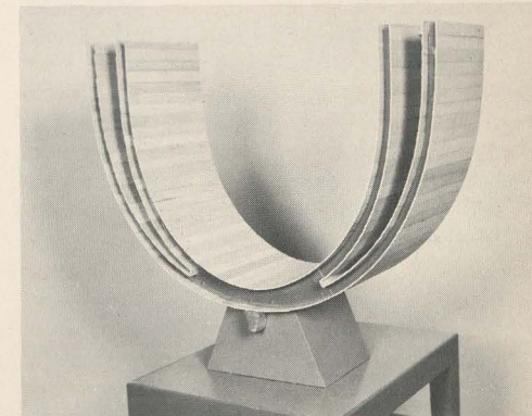
DOUBLE HULL FOR A SHIP. This practical idea provided safety for ships in time of war, so that if the enemy damaged its outer hull the inner one would keep it afloat. (Model of invention of Leonardo da Vinci)
