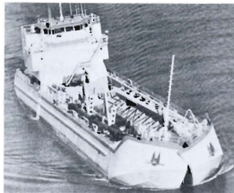
With her hull open to the sea, the Atchafalaya, smallest of the split-hull dredges, is shown here as she appears while dumping. The single dragarm is shown cradled beneath its davits on the starboard side of the hopper on the main deck.
